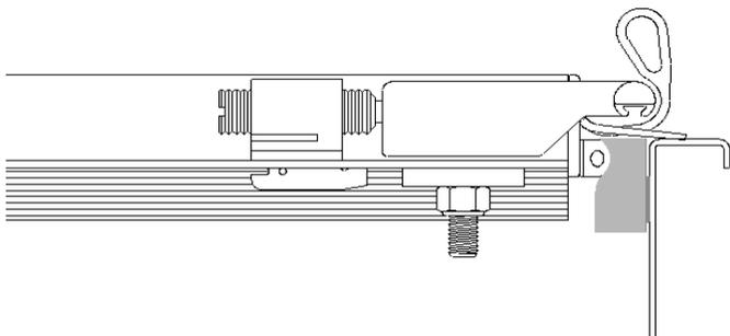
**STEP 3:** Side Rail Clamps: If your pickup bed does not have Utili-track channels, install three clamps on each side rail as shown in owner's Manual. If your pickup bed does have Utili-track channels, install two clamps on each side rail, locating clamps at each end of Utili-track channels.
