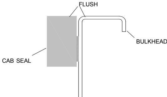
**STEP 2:** Side Rails: Position side rails against cab weather seal as shown below. See Owner's Manual for complete instructions.
