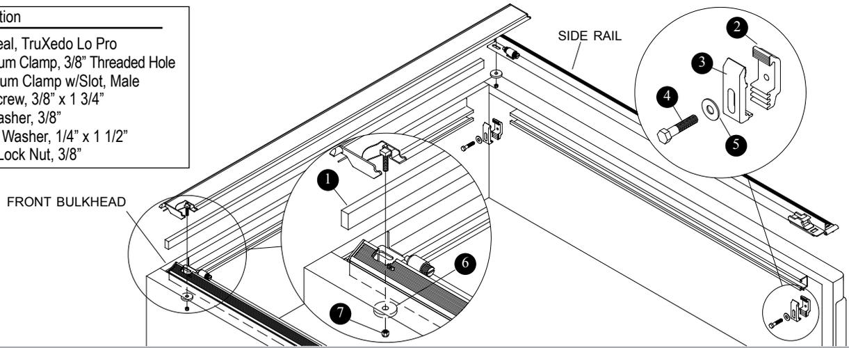
Follow these instructions to install cab weather seal, side rail clamps, and cab header on your 2005 or newer Nissan Frontier pickup. Refer to Owner's Manual for complete installation instructions.
